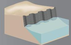
**BULKHEAD -** Vertical wall parallel to the shoreline intended to hold soil in place. Suitable for areas highly vulnerable to storm surge and wave forces.
