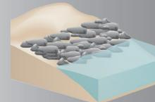
**REVETMENT -** Lays over the slope of the shoreline and protects it from erosion and waves. Suitable for sites with pre-existing hardened shoreline structures.
