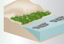
**BREAKWATER (vegetation optional) -** Offshore structures intended to break waves, reducing the force of wave action, and encourage sediment accretion. Suitable for most areas.
